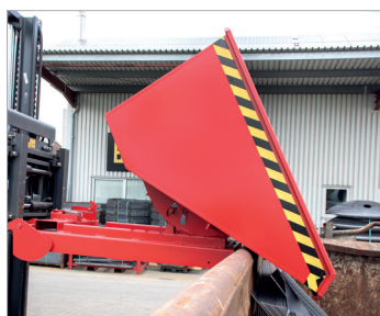
Emptied by activating release point 1
