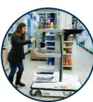
Very light overall weight of the unit ONLY 617 lbs 280 Kg makes it easy and comfortable to be pushed around and able to be used on every floor, even mezzanine floor.
